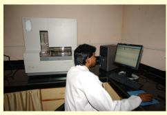
**Speed Vac** - Savant DNA 120 Speed Vac concentrator for concentrating of DNA & Proteins.
