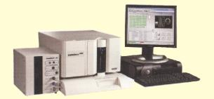
**5 Part Differential Blood Cell Counter** (model xt2000i) - for 28 different hematologic parameters including reticulocyte count.
