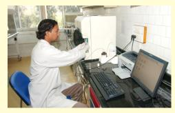
Real-Time PCR (LightCycler 480) - High-speed, high-accuracy Real-Time PCR (LightCycler 480) for gene expression analysis for various gene of parasite and host & genetic variation analysis with meltcurve and high-resolution melting (HRM).
